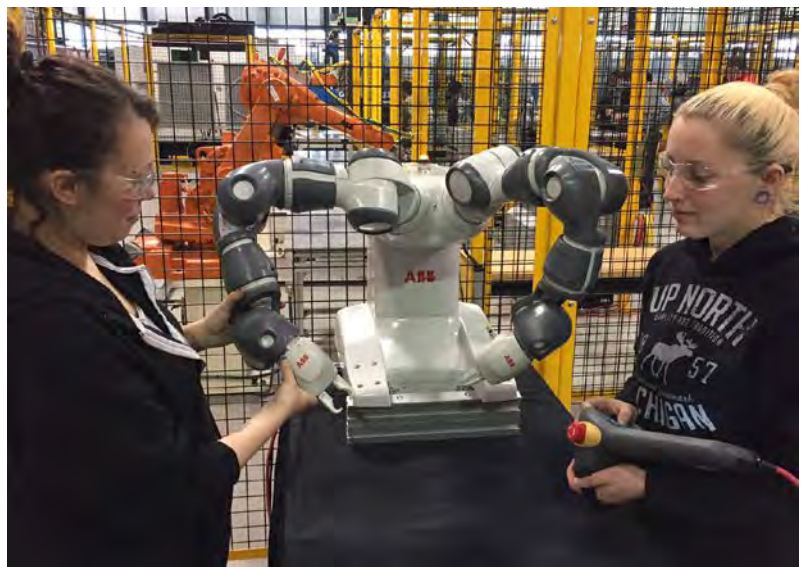
Students work on the new ABB Yumi robot purchased for the engineering technology lab.
