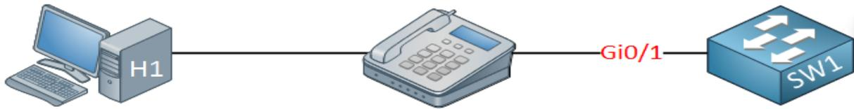
Cisco IP phones have a three-port switch inside of the IP phone:
